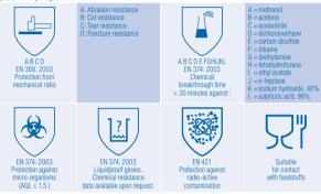
Warning! The information given in the pictograms or data provided on chemical resistant breakthrough times is based on lab tests and is therefore advisory only since it does not necessarily reflect the actual duration in the workplace. EC-Type examination certificate from Centextel Belgium (I.D. 0433), Technologiepark 7, B-9052 Zwijnaarde. For more detailed information on the glove's performance and to obtain a copy of the Conformity Declaration, please consult Anseli.
